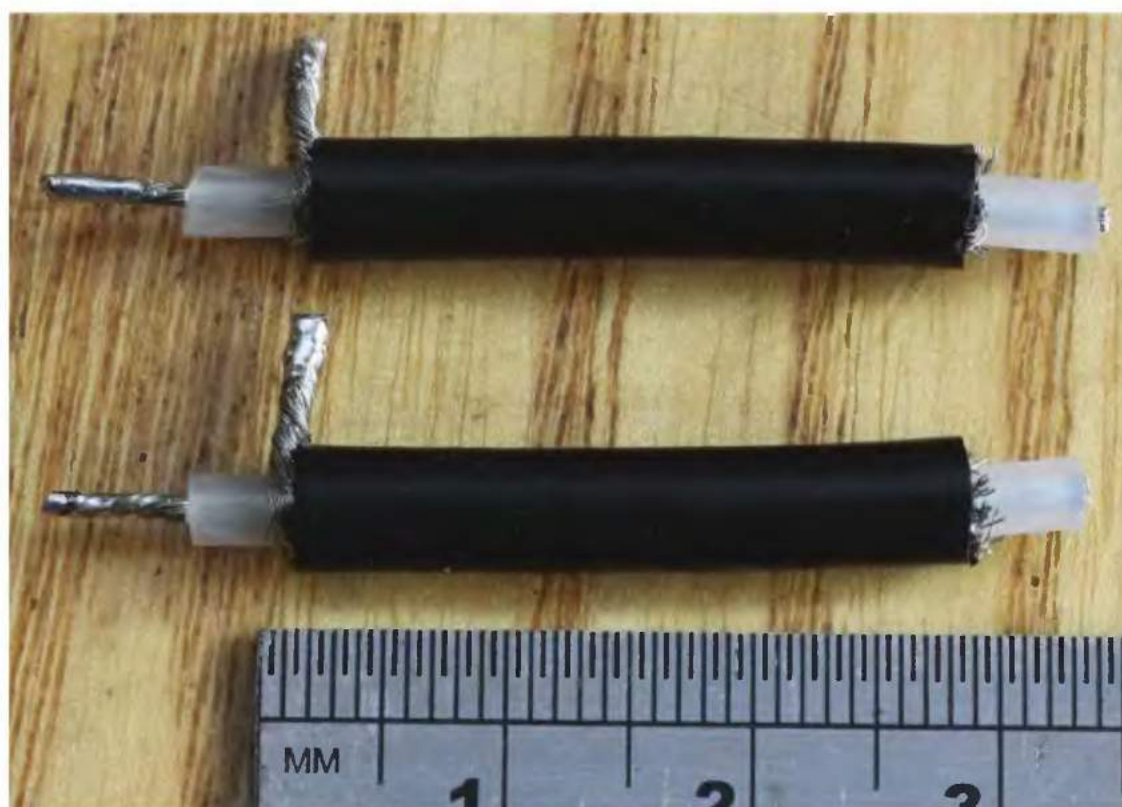
PHOTO 4: High voltage 3pF capacitors made from about 3cm of RG58 cable (see text).
