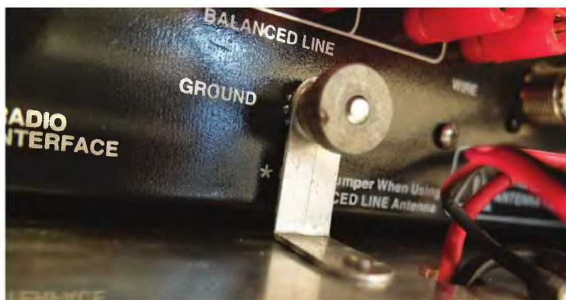
PHOTO 1: Earth terminal at rear of MFJ Intellituner.
