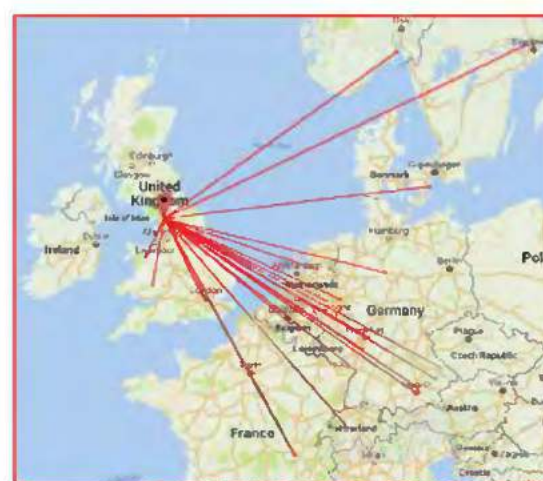
FIGURE 1: WSPR transmissions on 7MHz from 100m underground were received in 9 countries. Map Data ©2016 Geo-Basis/DE-BKG (©2009), Google Inst. Geogr. Nacional.
