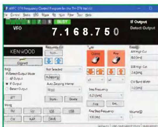
FIGURE 7: Controlling the TH-D74E using the ARFC-D74 frequency control program.
