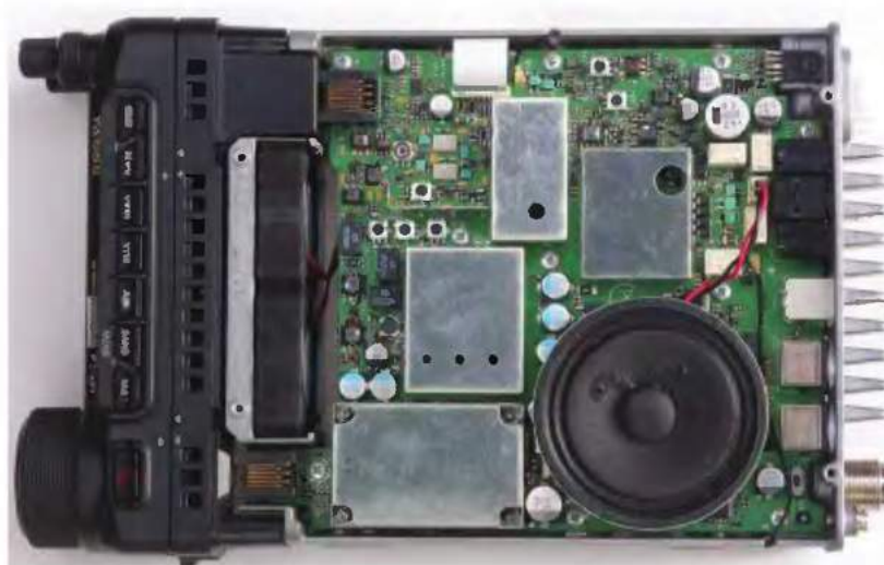
FT-891 Under the top cover showing signal processing board.
