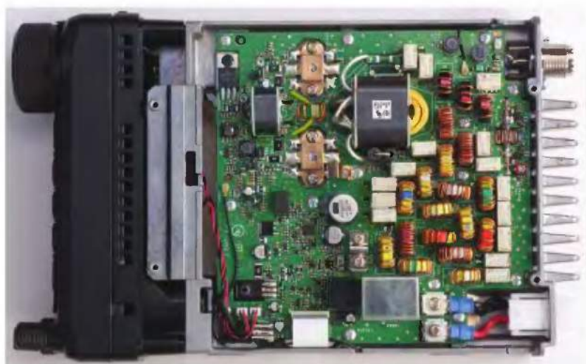
FT-891 Under the bottom cover showing power amplifier and filters.
