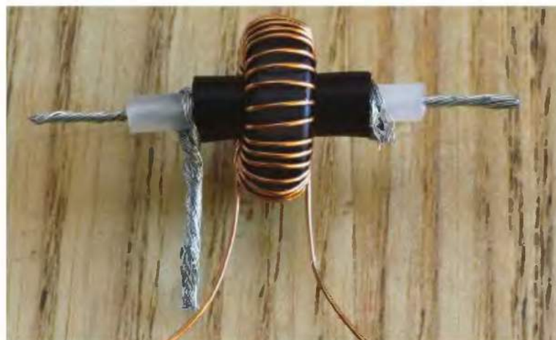
PHOTO 2: Practical configuration of a non-directional coupler.
