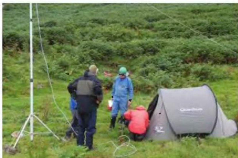
While barely practical underground, an inverted-V dipole is the antenna of choice on the surface.
