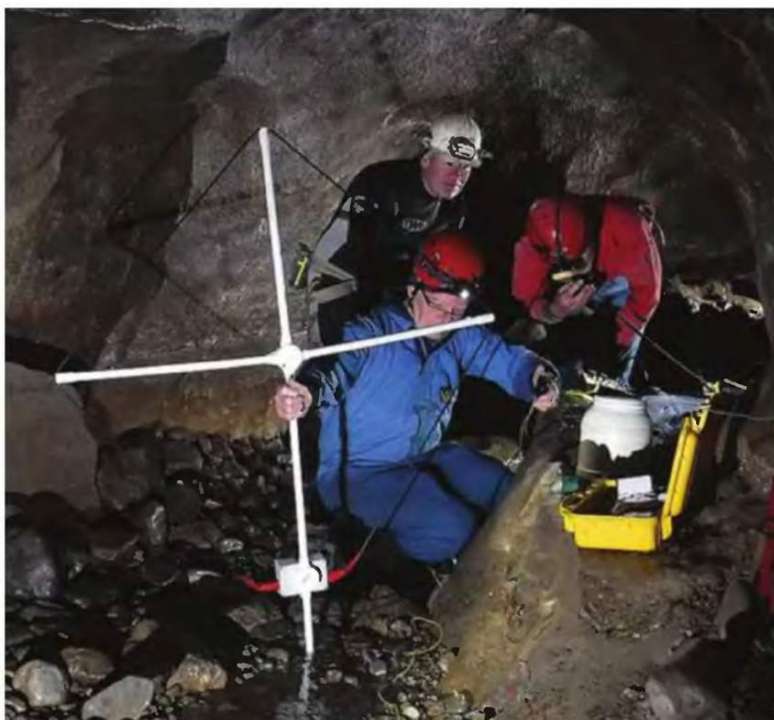
Loop antennas are a much more practical proposition than dipoles underground. (Photo: Gregory Collins).
